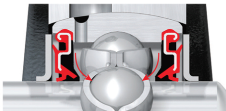
Fig. 3: New seal design for lubrication
